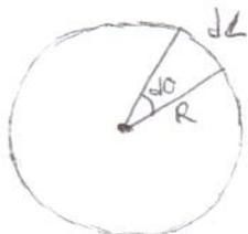
$$dL = R d\theta \quad \text{con } d\theta \text{ in radianti}$$
