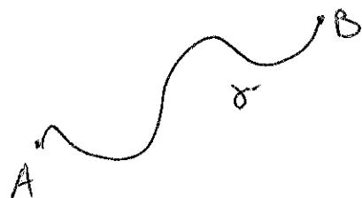
$$\begin{aligned} L_\gamma(A \rightarrow B) &= \int_{\gamma} \vec{F} \cdot d\vec{s} \\ &= \int_A^B [F_x dx + F_y dy + F_z dz] \end{aligned}$$
