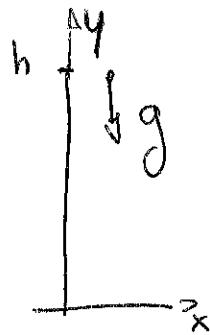
$$\begin{aligned} & \left\{ \begin{array}{l} y = y_0 + v_0 t - \frac{1}{2} g t^2 \\ v = v_0 - g t \end{array} \right. \\ \downarrow & \left\{ \begin{array}{l} 0 = 3m - \frac{1}{2} 9,8 t^2 \rightarrow t = 0,783 s \\ v = - 9,8 \frac{m}{s^2} \cdot 0,783 s \\ = 7,67 \frac{m}{s} \end{array} \right. \end{aligned}$$
