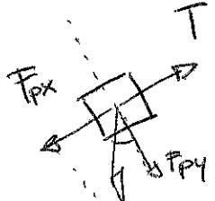
$$\begin{aligned} T &= F_{px} = F_p \sin \theta \\ &= mg \sin \theta \end{aligned}$$
