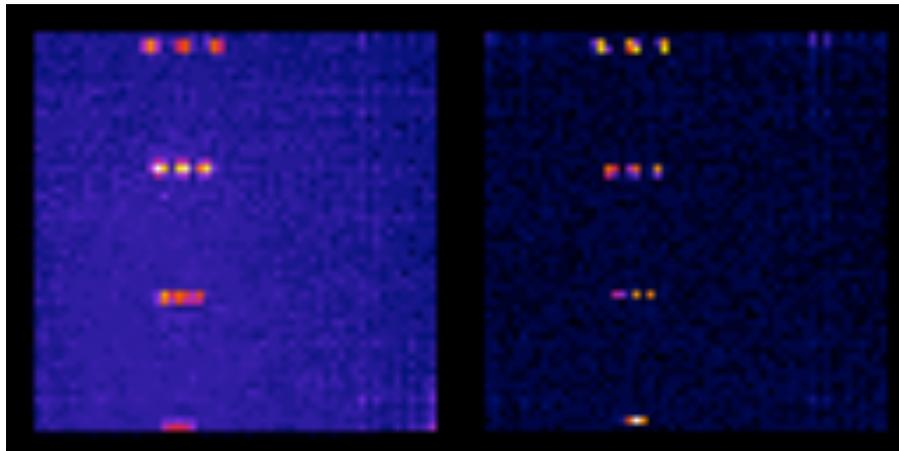
**Figure 6.** 2-D images acquired illuminating a sensor through the Pb mask above described with  $^{57}\text{Co}$  (left) and  $^{241}\text{Am}$  (right).
