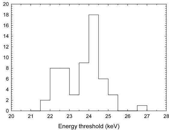
**Figure 4.** Energy threshold distribution of a silicon detector
