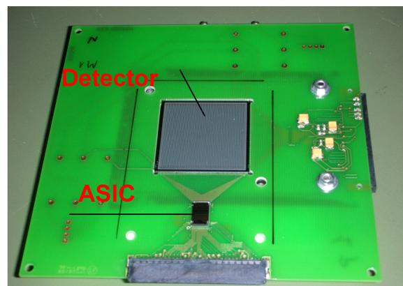
**Figure 1.** Schematic drawing of the SiliPET scanner. **Figure 2.** Photo of the PCB support developed by INFN-Ferrara.
