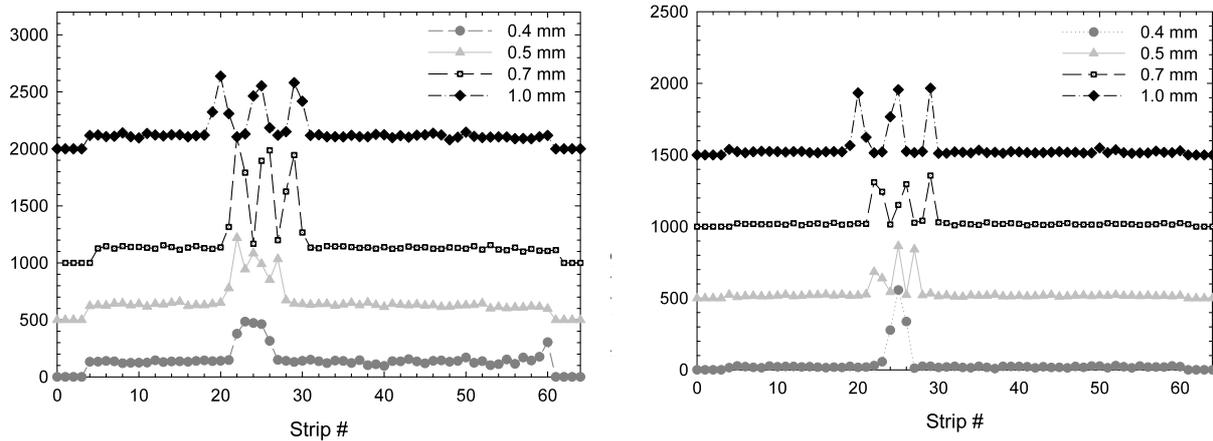
**Figure 7.** Horizontal profiles of the 2-D images illustrated in Fig. 24:  $^{57}\text{Co}$  (left) and  $^{241}\text{Am}$  (right). The distributions are intentionally shifted along the vertical axis to obtain a more readable graph.
