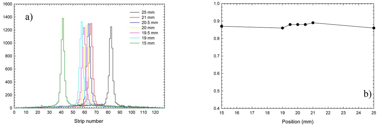
**Figure 3.** a) Profiles acquired at different positions, b) Spatial resolution measured with a 1 mm diameter  $^{22}\text{Na}$  source.
