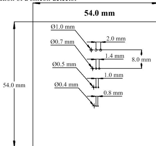
**Figure 5.** Schematic drawing of the Pb mask used to evaluate the spatial resolution.
