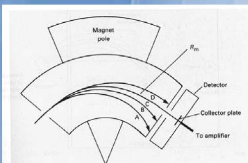
Fig. 11.25. Representative of ion generation between acceleration plates. Only ions following a trajectory of radius  $R_m$  will be focused. A, B and D are currently defocused. By altering the field, other ions can be forced to travel along  $R_m$  and be focused.
