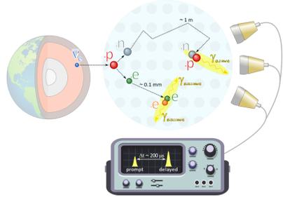
**KamLAND** is a **1 kton** liquid scintillator detector situated in the Kamioka mine. It is surrounded by 1325 17" PMTs and 554 20" PMTs.
