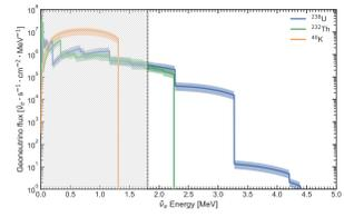
Uranium (U) and thorium (Th) geoneutrinos are detected via **Inverse Beta Decay** on free protons inside big **liquid scintillator detectors**. The measurement of the geoneutrino **flux at surface** permits to estimate the U and Th content of our planet's mantle and in turn to derive its **radiogenic heat production**.
