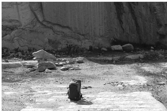
Fig. 1 – Portable gamma-ray spectrometer in a quarry during the acquisition of K-U-Th isotopic concentration.
