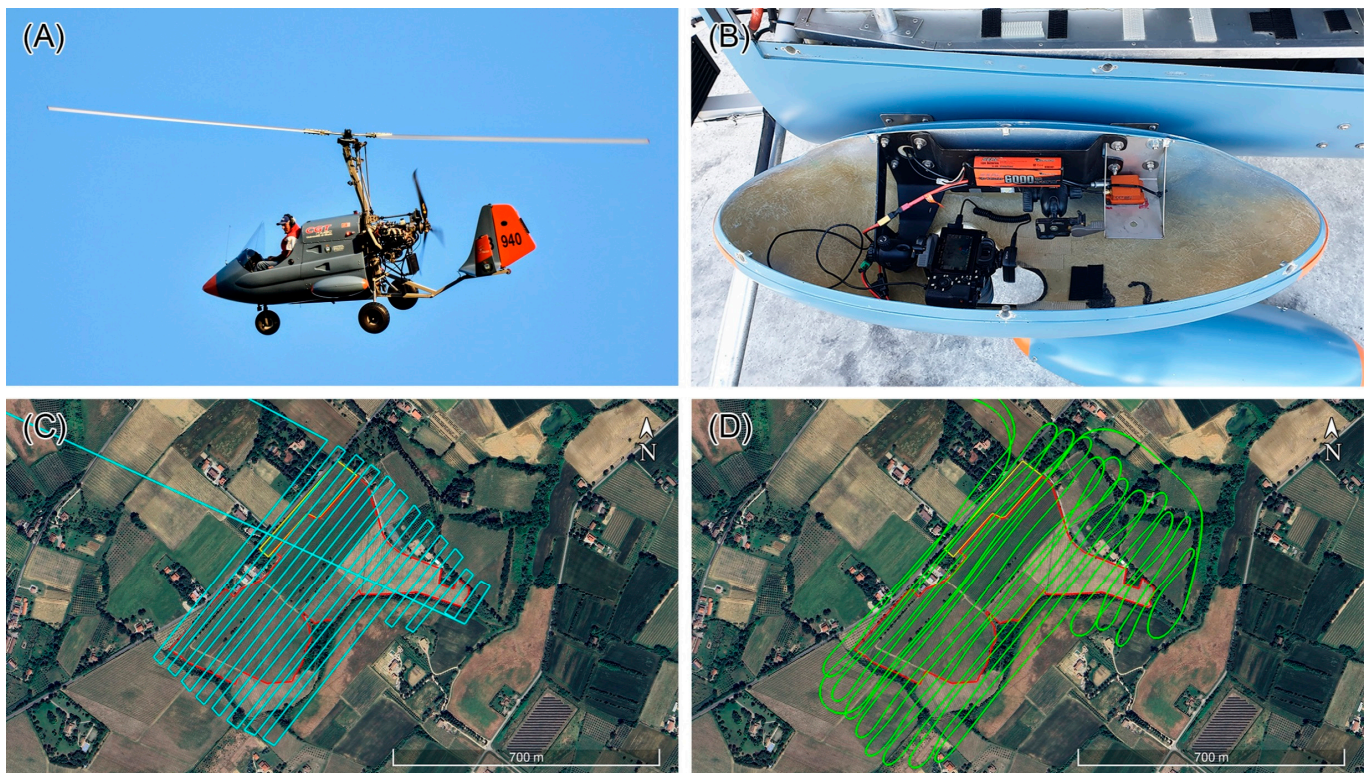
Figure 2. (A) Radgyro, the aircraft used for the airborne photogrammetric survey. (B) The camera and independent alimention system installed in the lateral compartment of the Radgyro. (C) Flight plan and (D) flight path of the survey performed in the study area. The red and yellow lines delimit the portions of investigated vineyard cultivated, respectively, with red grapes and white grapes.
