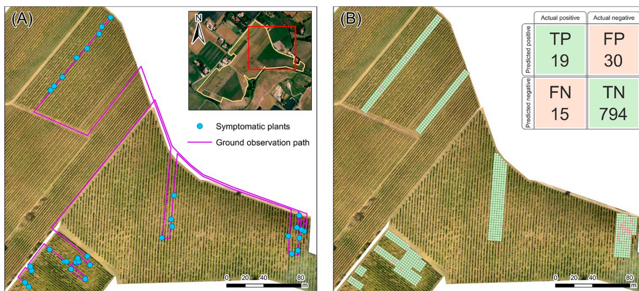
Figure 11. The area of the experimental site investigated through the field ground observation campaign. (A) Path followed and location of the plants with observed symptoms of grapevine yellows (FD and BN) and trunk disease (EC). (B) Spatial distribution of the Prediction Boxes (PBs) resulted in agreement (TP and TN) or in disagreement (FP and FN) with the ground observations.
