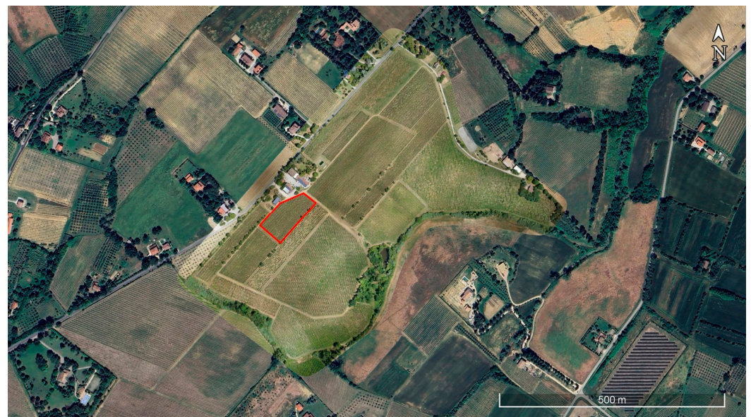
Figure 3. Georeferenced orthomosaic derived from the processing of the photograms acquired during the airborne survey performed in the study area. The red line indicates the sample parcel used for the identification and testing of the vegetation indices (see Section 2.3).
