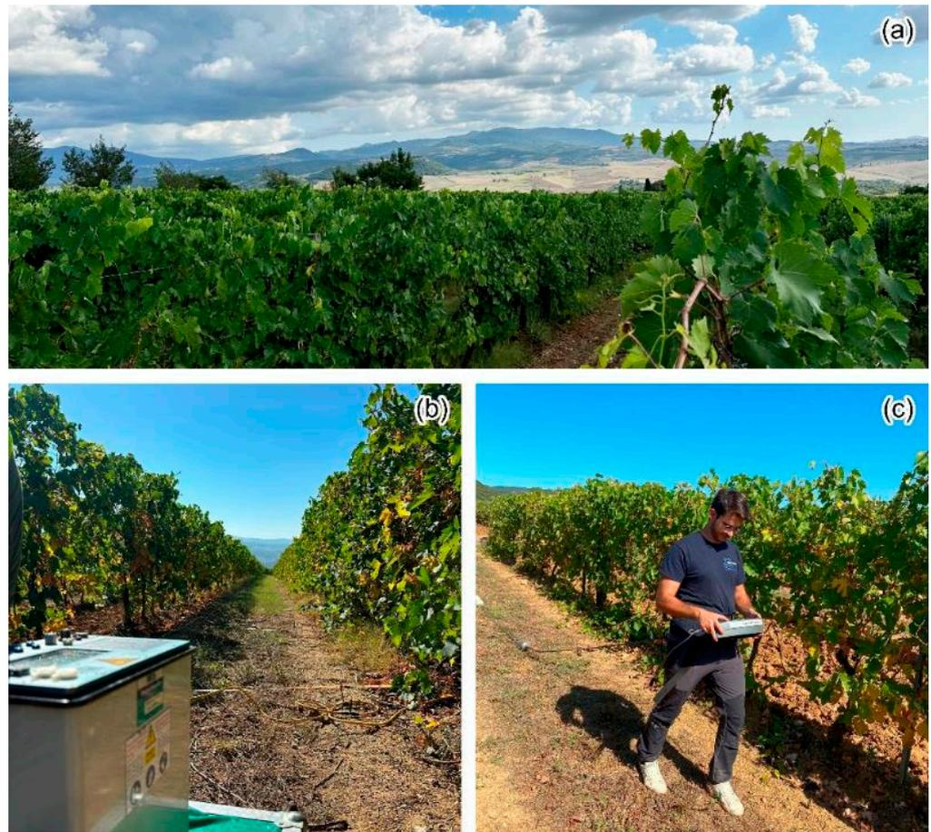
**Figure 2.** Data collection. (a) An overview of the study area. (b) The Syscal Pro instrument used in the GCR method. (c) A field operator using the OhmMapper for CCR measurements.
