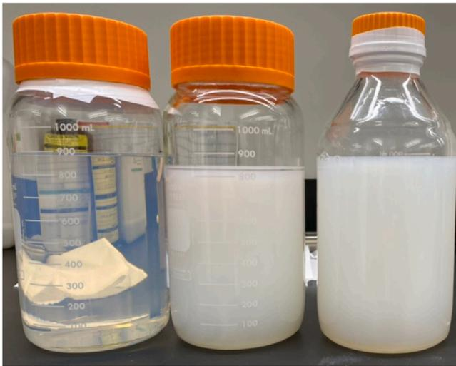
**Fig. 3.** From left to right: oWbLS1, oWbLS2, oWbLS3. oWbLS1 has the longest scattering length of the three oWbLS samples and appears relatively transparent, and oWbLS2 has the shortest scattering length.
