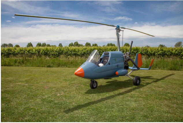
Fig. 1. Picture of the Radgyro, the autogyro dedicated to multispectral airborne acquisitions, used for the AGRS surveys over the sea.
