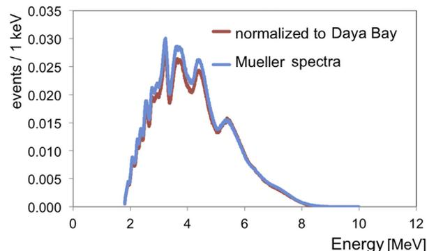
**Fig. 2.** Reactor antineutrino spectra expected in Borexino, assuming 100% efficiency in the period December 2007 - October 2017, with Mueller spectra (blue) or with the normalization to the Daya Bay measurement (red). (For interpretation of the references to colour in this figure legend, the reader is referred to the web version of this article.)
