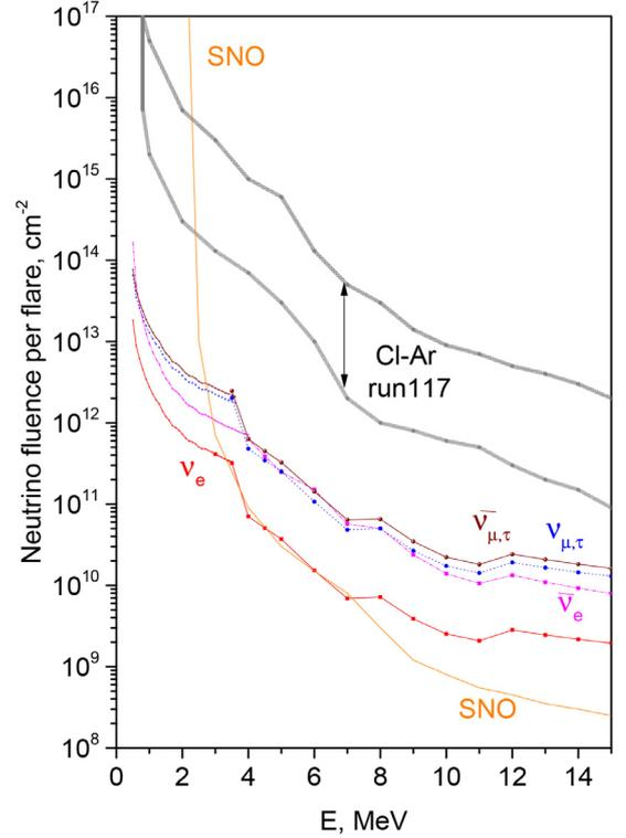
**Fig. 8.** Borexino 90% C.L. fluence upper limits obtained through neutrino-electron elastic scattering for  $\nu_e$ ,  $\bar{\nu}_e$ ,  $\nu_{\mu,\tau}$ , and  $\bar{\nu}_{\mu,\tau}$ . In the plot the limits obtained for  $\nu_e$  by SNO [16] are labelled and the range of fluences that would have explained the Cl-Ar Homestake excess in run 117.
