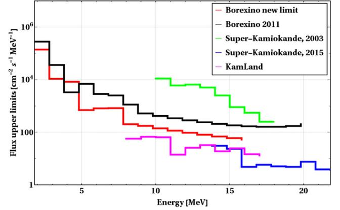
**Fig. 4.** New Borexino model-independent limits on electron  $\bar{\nu}_e$  fluxes from unknown sources in comparison with the results of other detectors (Super-Kamiokande [51,52], KamLAND [18]) and previous Borexino limits [21].
