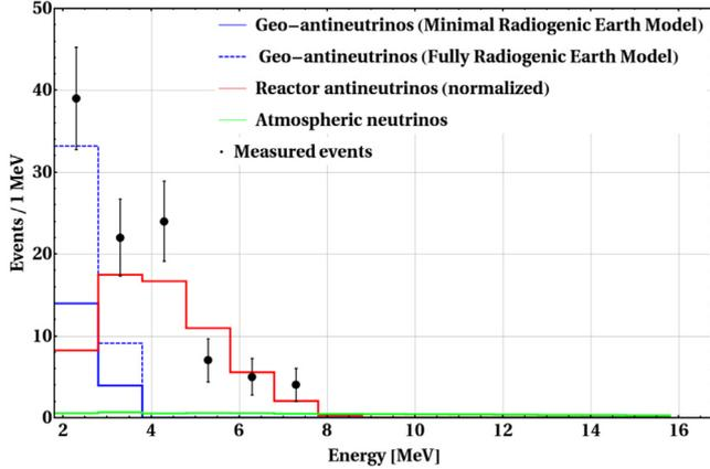
**Fig. 3.** The number of measured events (black data point) is compared for each energy bin with the expected backgrounds (red – reactor  $\bar{\nu}_e$ , green – atmospheric  $\nu$ , blue – geo- $\bar{\nu}_e$  according to Minimal Radiogenic model, dashed blue – geo- $\bar{\nu}_e$  according to Maximal Radiogenic model, see text for details). (For interpretation of the references to colour in this figure legend, the reader is referred to the web version of this article.)
