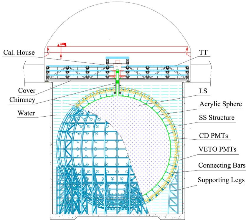
Fig. 3. Schematic view of the JUNO detector.
