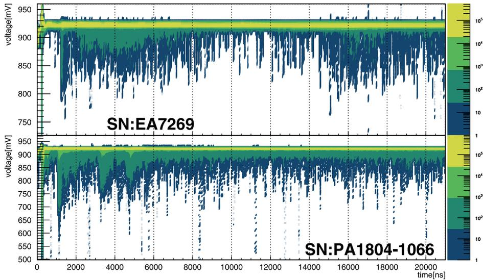
**Fig. 21.** Two dimensional plot of the afterpulse waveforms, for a dynode PMT with serial number of EA7269 (upper) and a MCP PMT with serial number of PA1804-1066 (lower).
