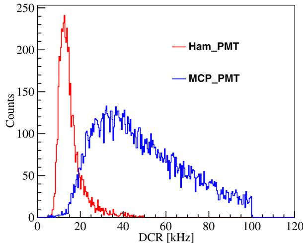
Fig. 20. DCR distributions for MCP PMTs and dynode PMTs.
