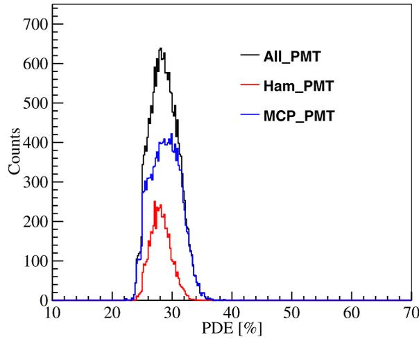
Fig. 19. PDE distributions for all PMTs, MCP PMTs and dynode PMTs.
