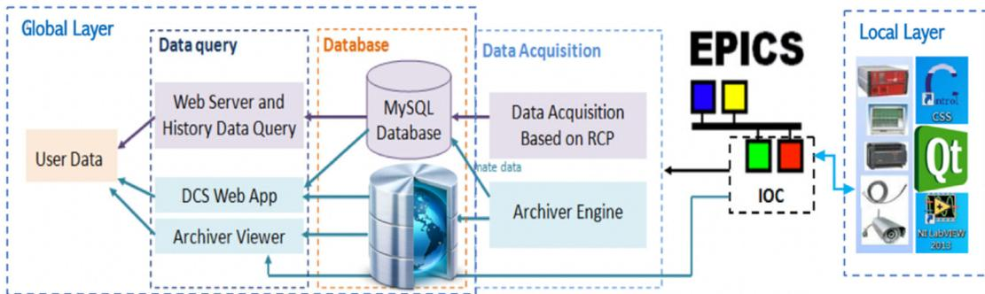
**Fig. 29.** Scheme of the Detector Control System. The DCS framework is based on EPICS and is divided into the Local Layer, the Data Acquisition Layer, and the Global Layer. The Local Layer includes the firmware of the embedded devices and the Industrial PCs. The Data Acquisition Layer reads data from IOCs and save it into the databases. The Global Layer includes the databases and the user interfaces.
