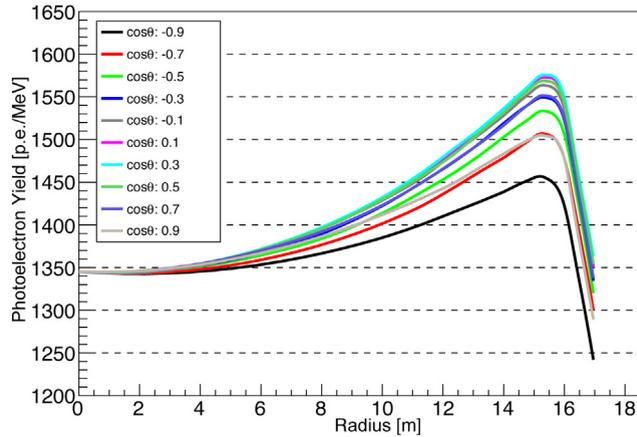
Fig. 30. Mean number of photoelectrons per MeV for 2.22 MeV gammas as a function of radius at representative polar angles.
