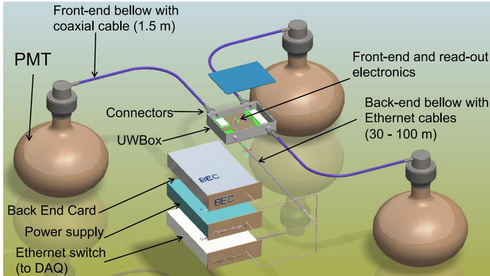
Fig. 24. Large PMT electronics technical drawing.
