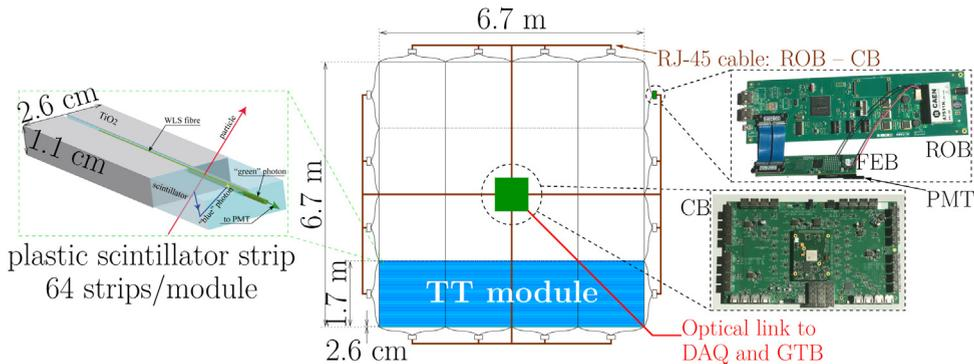
Fig. 14. Schematics of a TT wall, with detail of a plastic scintillator strip (left), and photos of the TT wall electronics (right). Dimensions of a TT wall, a TT module (one of the modules is shown in blue) and a plastic scintillator strip are also drawn.
