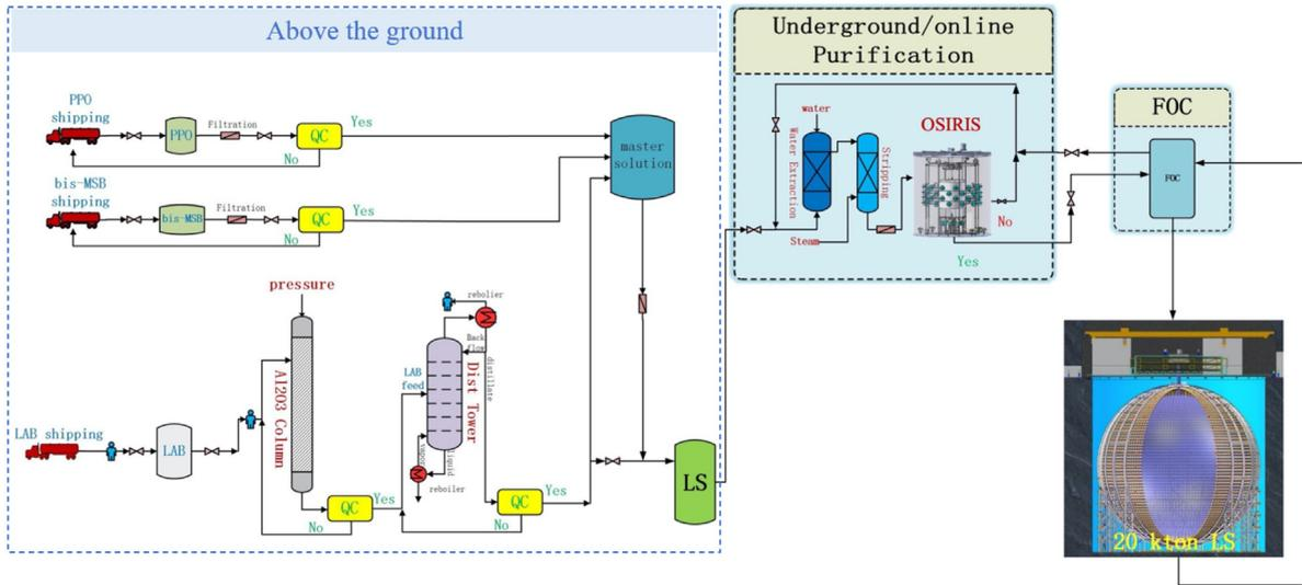
Fig. 15. Flowchart of the liquid scintillator processing system.
