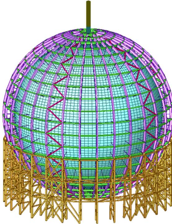
**Fig. 11.** Scheme of the Central Detector (CD). The spherical Acrylic Vessel is supported by a spherical stainless steel shell structure via 590 Connecting Bars. The shell structure sits on a bearing consisting of 30 pairs of Supporting Legs made of stainless steel truss structures.
