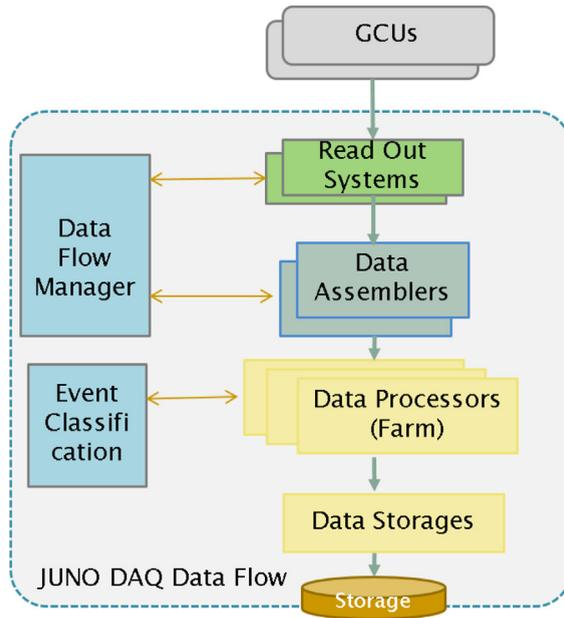
**Fig. 28.** The DAQ data flow consisting of four levels of scalable and distributed data processing including the readout systems, data assemblers, data processors, and data storages, and two centralized data processing including the data flow manager and the event classification.
