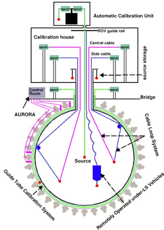
Fig. 27. Overview of the calibration system (not drawn to scale).
