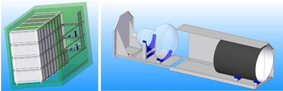
**Fig. 17.** *Left:* Conceptual picture of the container with the shelf system including 36 drawer boxes. *Right:* Schematic view of the final design of the drawer system (for illustrative reasons one side of the drawer box is not depicted).
