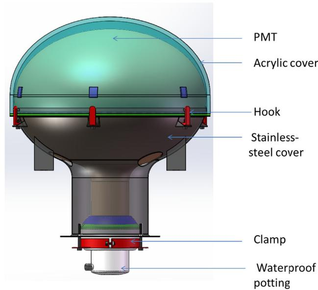
Fig. 22. Schematics of an instrumented MCP PMT.
