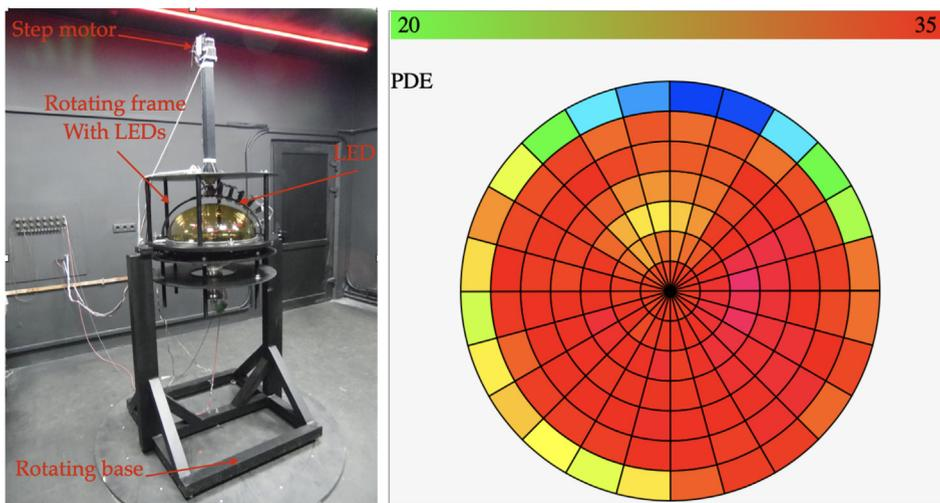
**Fig. 18.** 20-inch PMT scanning: left – Overall view of the scan station; right – Scanning map for a dynode PMT.
