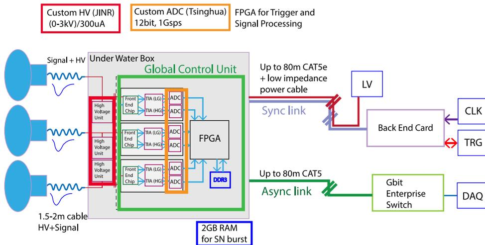
Fig. 23. Large PMT electronics scheme: the ‘wet’ electronics (left) is connected to the ‘dry’ electronics by means of Ethernet cables and a dedicated low impedance cable for power distribution.
