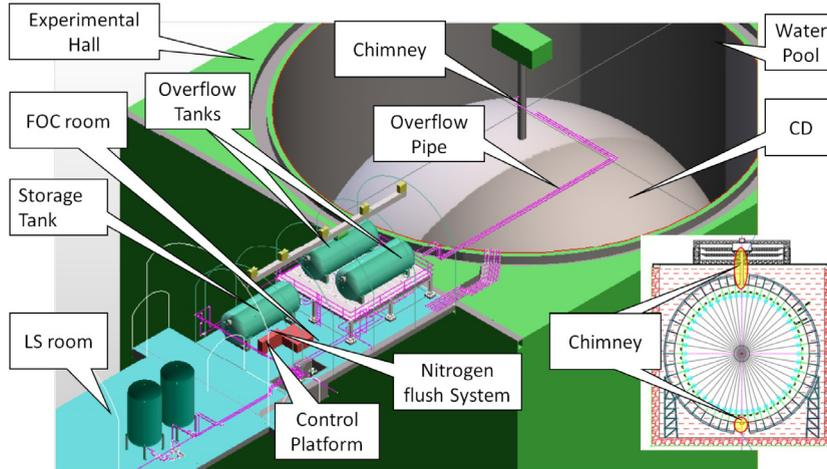
**Fig. 12.** Scheme of the Filling, Overflow, and Circulation (FOC) system.
