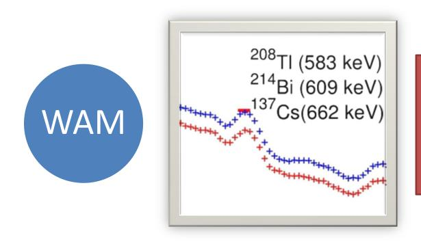
The Cava\_Rad Nal(Tl) does not resolve the triplet in energetic range of <sup>137</sup>Cs
