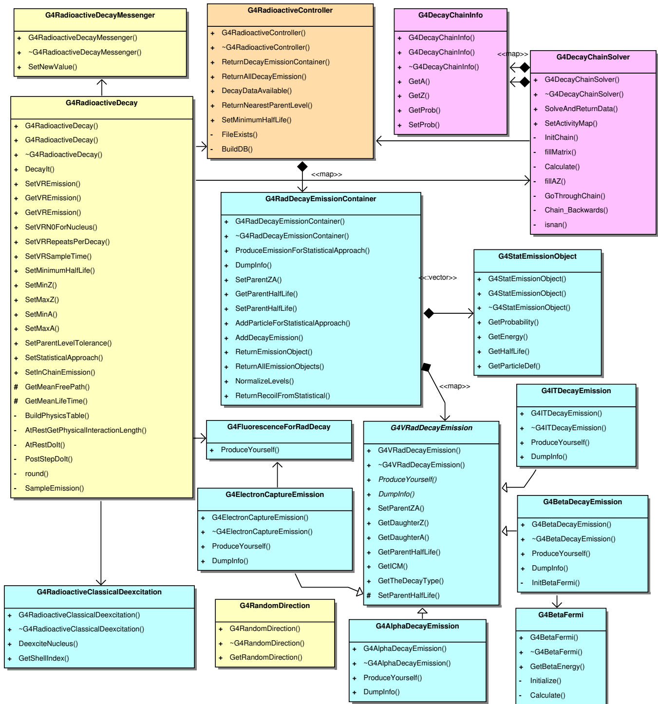
Fig. 3. A UML class diagram for the RDM-extended package implementing a refactored per-decay sampling and a statistical sampling method. The colors (grey shades) reflect the responsibilities and are matched to the activity diagram in Fig. 4: physics simulation (blue/medium grey), data management and preparation (orange/medium dark grey) and decay chain processing (purple/dark grey). Each decay type class is responsible for simulating the type's characteristic physics. The deexcitation and fluorescence emission for the statistical simulation approach is produced by the G4VDecayEmission base class.
