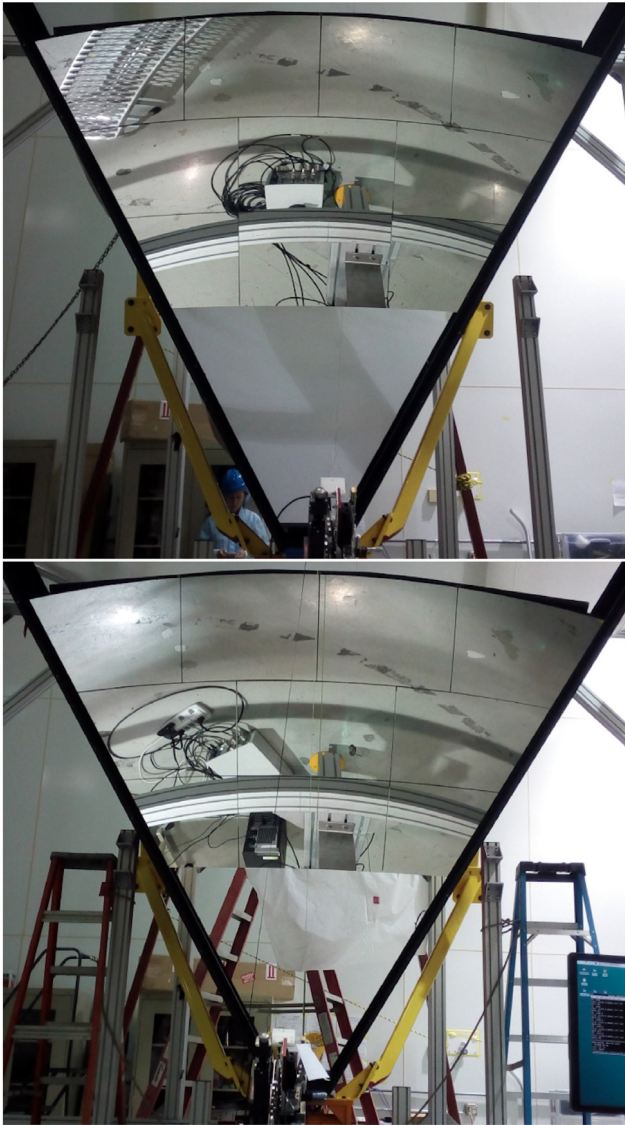
Fig. 18. The spherical mirror before (top plot) and after (bottom plot) alignment. As a result of the alignment, the image appears continuous along the whole mirror surface.
