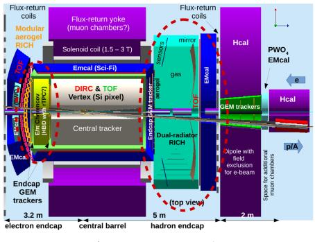
The JLab central detector concept includes a DIRC, a dual-radiator and a modular aerogel RICH detectors and a  $4\pi$  TOF for the PID. Three models of the EIC detector are under study at JLab and BNL, with slightly different layouts of the hadron identification. The PID consortium aims to develop an integrated solution useful for both BNL and Jlab.
