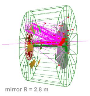
**Photo-detector**: spherical shape, 8500 cm<sup>2</sup> (per sector), pixel size 3 mm
