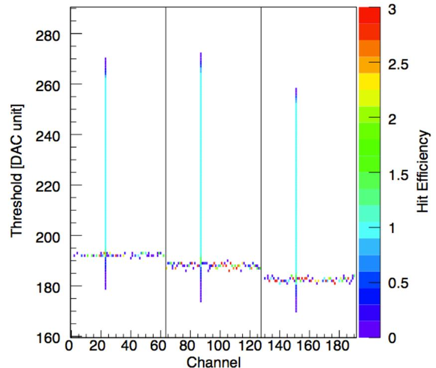
Discrimination down to 20 fC, i.e. few % of SPE, allows sensor characterization
