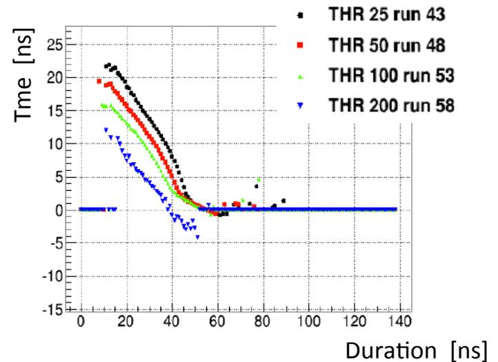
Channel by channel time calibration: no offsets
