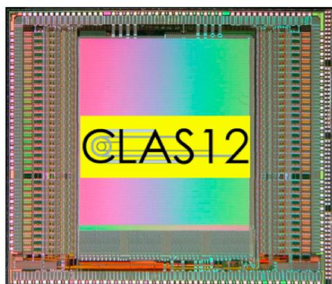
Single Channel (x64) - Design for Micromegas @ CLAS12
