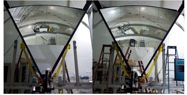
Figure 8: The spherical mirror before (left) and after (right) alignment.
