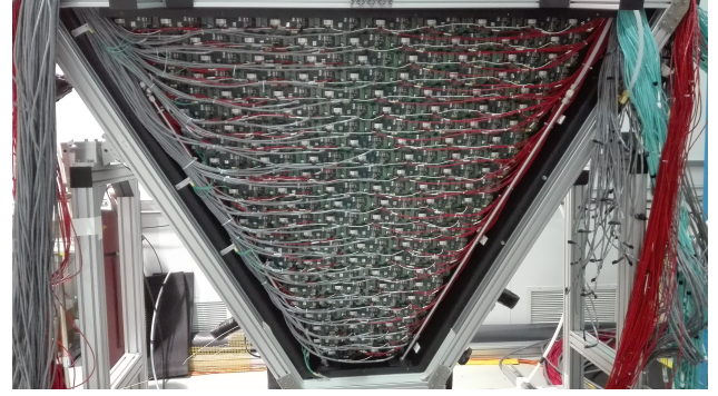
Figure 17: The Front End electronics fully assembled and cabled.
