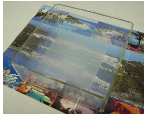
Fig. 8. Photograph of an aerogel with the frame structure. The aerogel with extremely low density looks white in the center. Density : 0.0088 \pm 0.0008 g/cm 3 Corresponding Refractive Index : 1.002 Size : 7 \times 7 \times 1 cm
