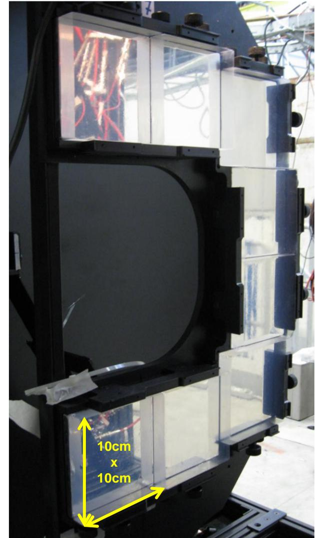
Radiator  $n=1.05$ ,  $t=6\text{cm}$ ; Beam  $p = 6\text{GeV}/c$ : Comparison with and without absorbers:
