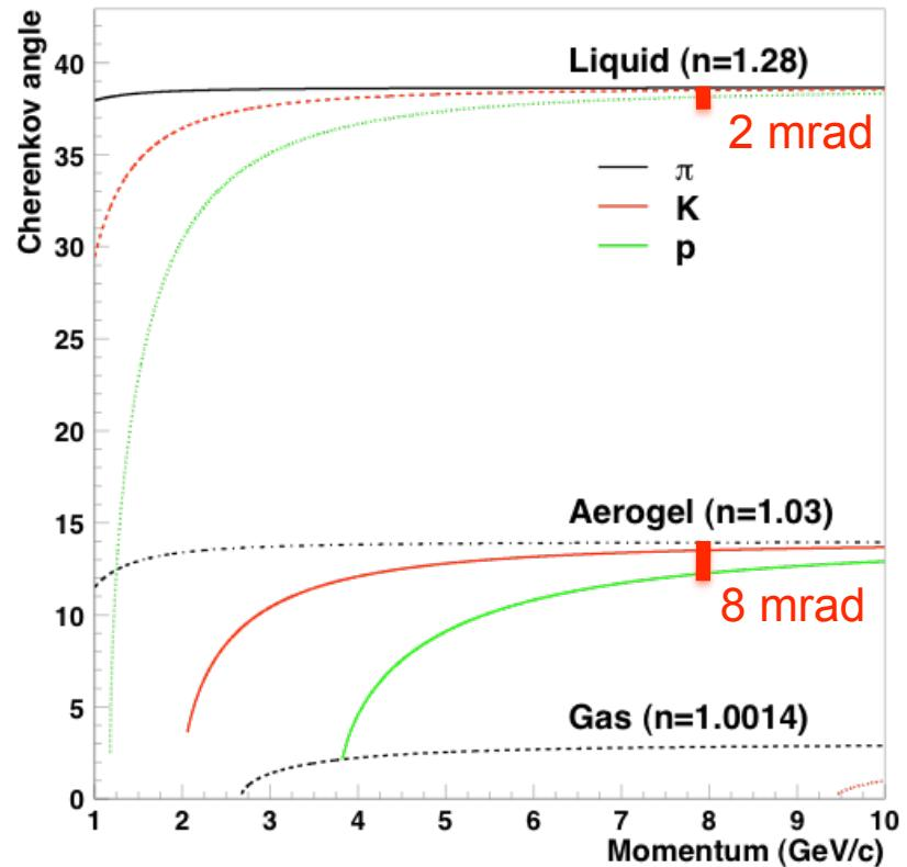
**Freon+UV-light detection** does not provide enough discrimination power in the 2-8  $\text{GeV}/c$  momentum range (chromatic dispersion) → no cheap solution
