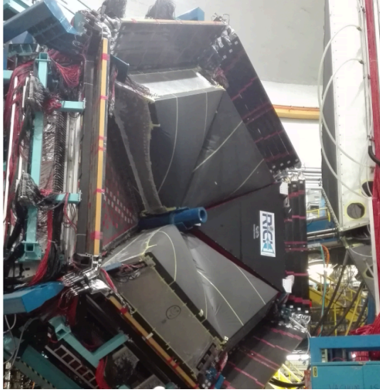
Figure 1: The first module of the CLAS12 RICH installed in Sector 4 of the Hall B Forward Carriage.
