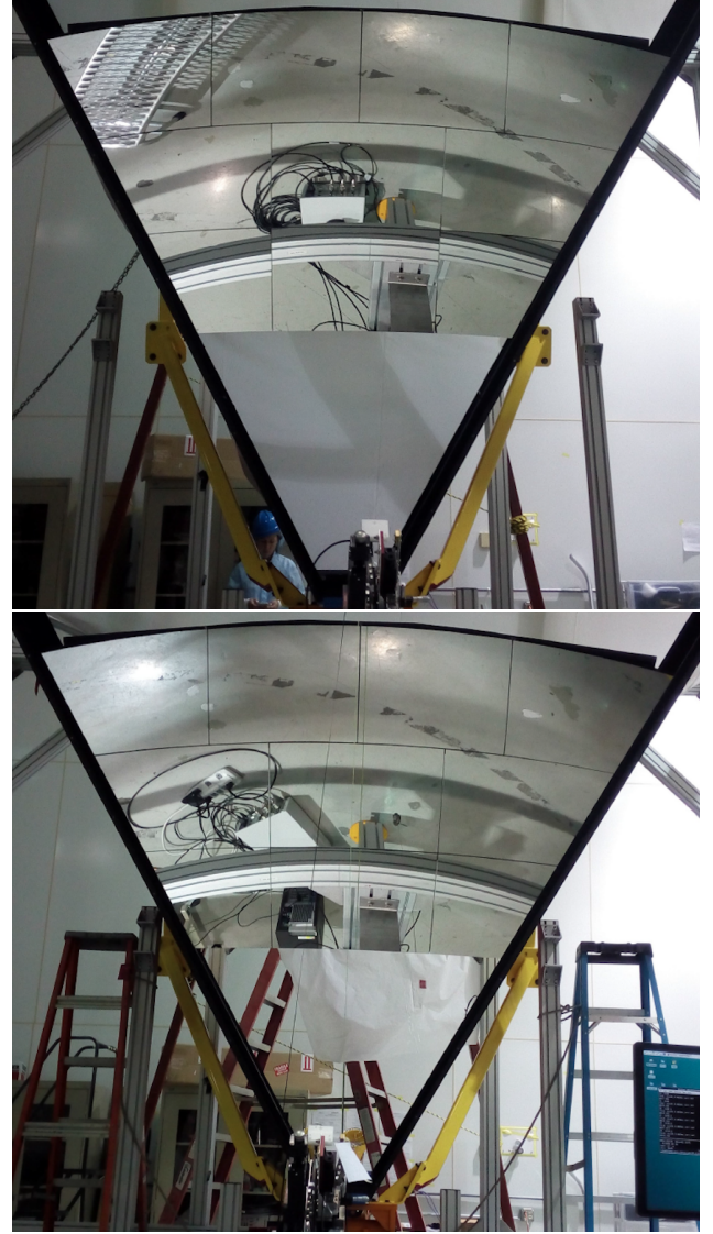
Figure 18: The spherical mirror before (top plot) and after (bottom plot) alignment. As a result of the alignment, the image appears continuous along the whole mirror surface.
