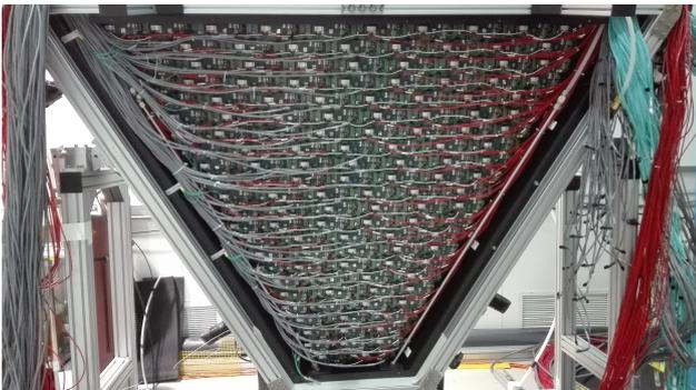
Figure 21: The fully assembled and cabled front-end electronics. Visible are the gray 20 AWG LV cables, the red HTC-50-1-1 HV cables, and the cyan MTP<sup>540</sup> optical fibers.
