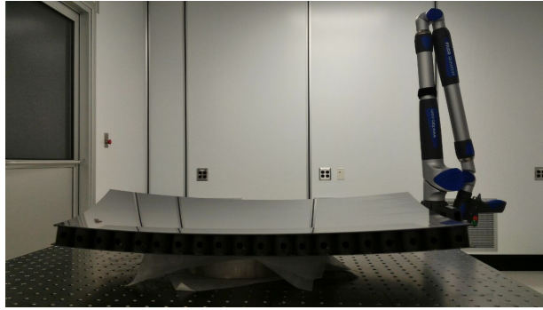
Figure 7: Mirror leaning on the cylindrical support, awaiting to start the CMM operations.
