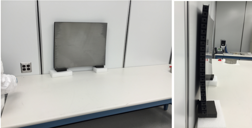
Figure 3: Mirror in vertical position for spot-image measurement.
