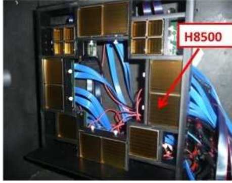
Figure 23: The photo-detection area of the RICH prototype used at the test beam at CERN.
