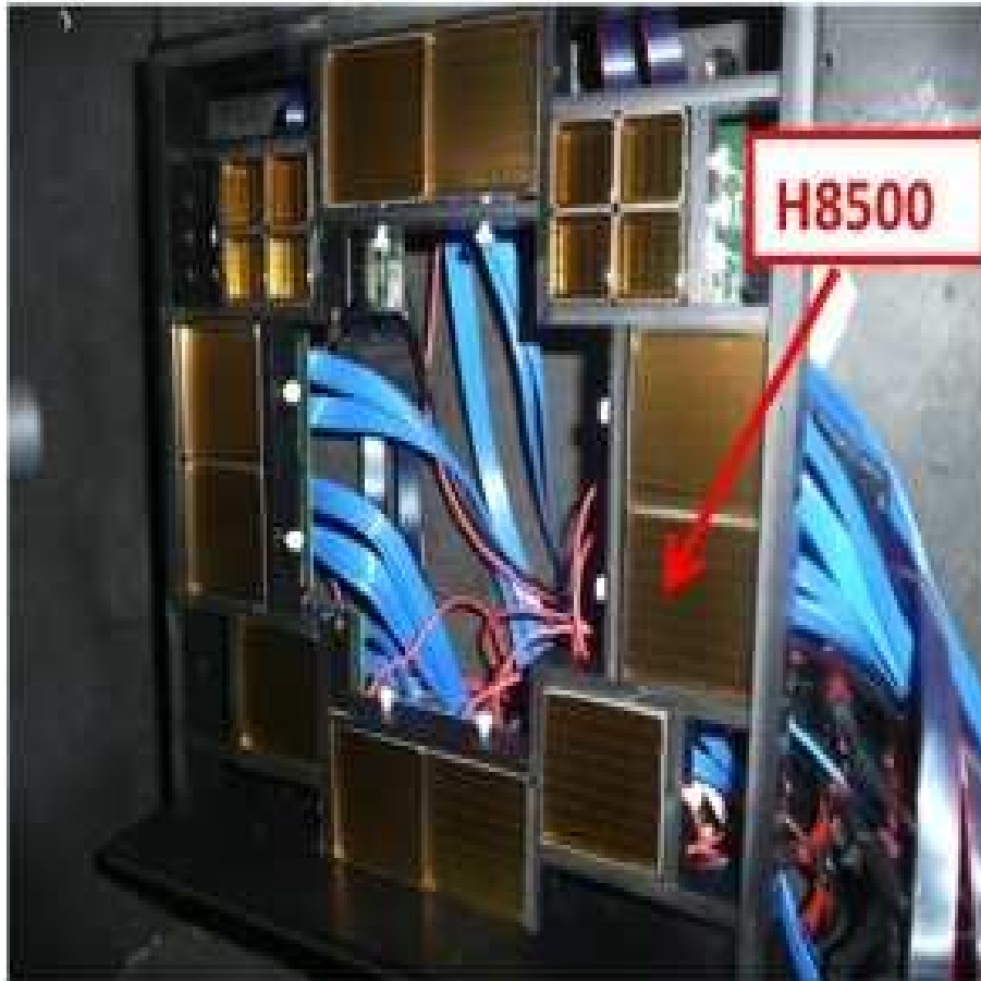
Figure 23: The photo-detection area of the RICH prototype used at the test beam at CERN.
