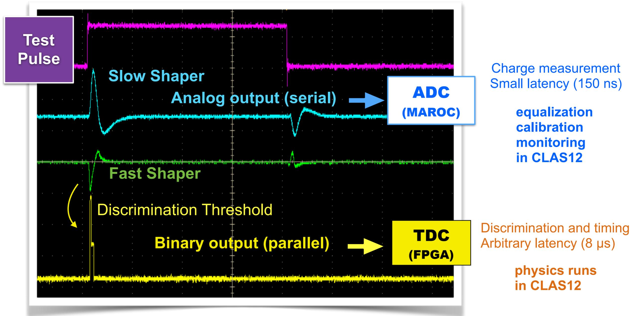
external, internal + **self triggered** data acquisition
