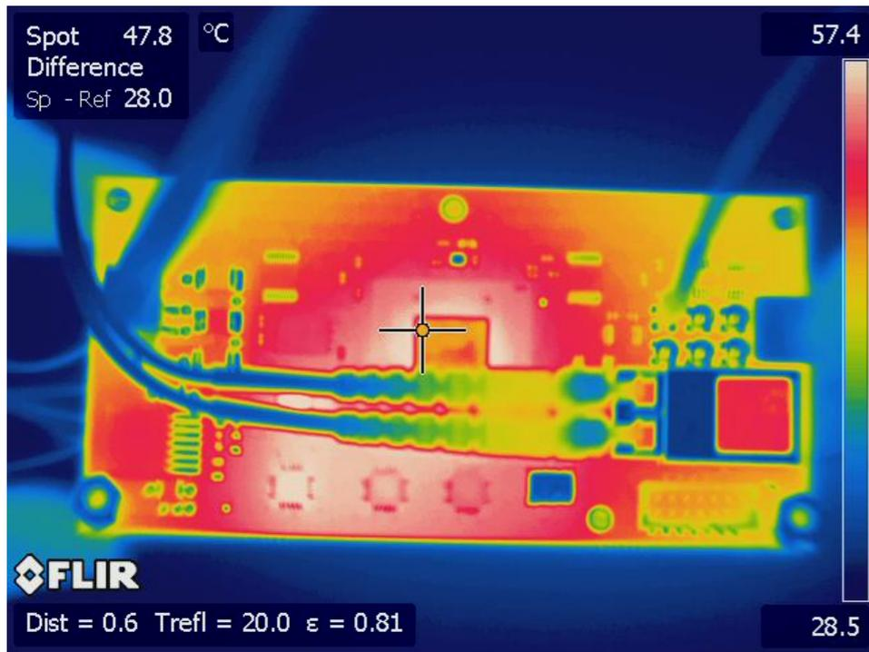
Majority of the heat is produced by the FPGA board
