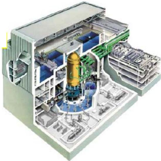
**ABWR (Advanced Boiling Water Reactor)**
