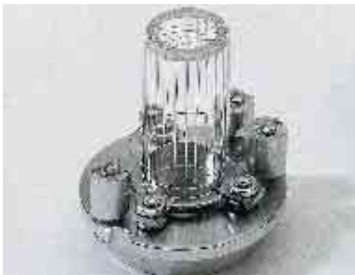
Fig. 12: Grid ion source for extreme ultra high vacuum measurements.
