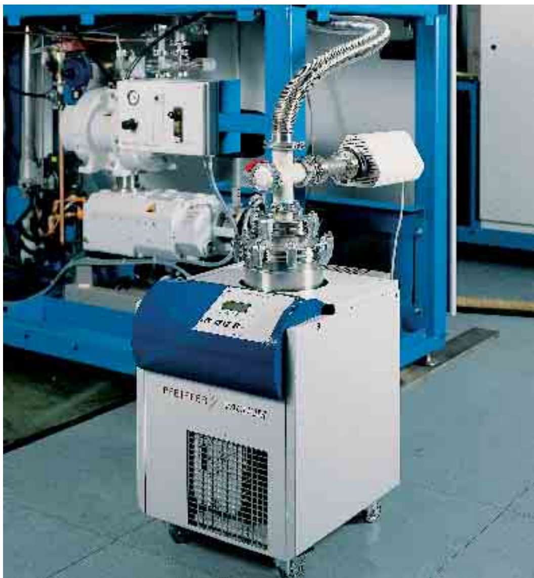
Fig. 37: Monitoring of gas composition on production system.
