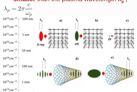
**Acceleration** in a **nanostructure** (crystal or carbon nanotube) **limits scattering** off the solid's ions.
