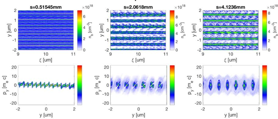
Don't need a small driver! Imprint the target structure on the drive beam
