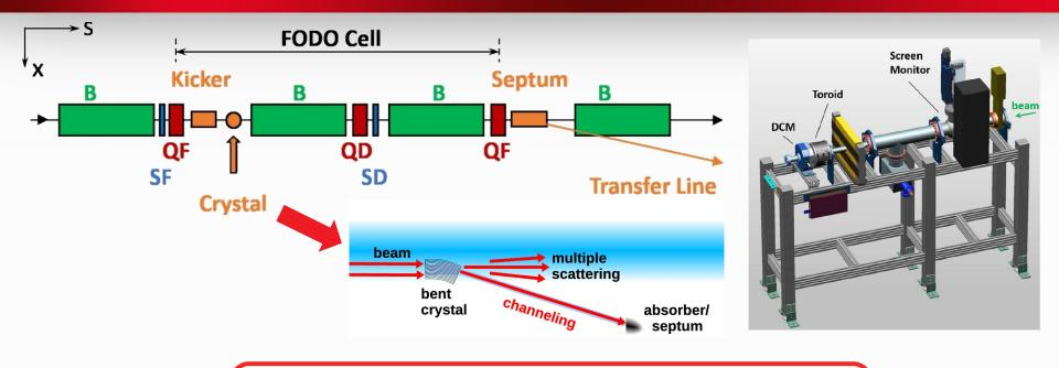
Crystal-based beam extraction: applied only for protons, never applied for electrons
