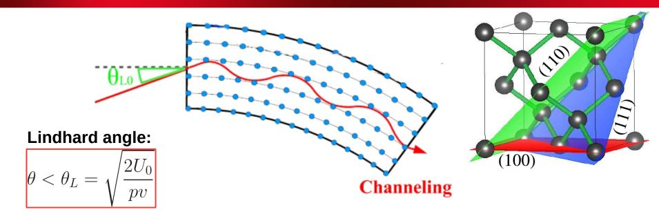
Channeling\* is the effect of the penetration of charged particles through a monocrystal quasi parallel to its atomic axes or planes. In dependence on the crystal alignment along either planes or atomic strings channeling can be divided into
