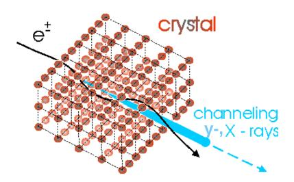
Coherent effects preserve **up to few mrad** of particle direction vs the crystal axis
