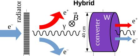
Coherent effects in a crystal accelerate electromagnetic shower development
