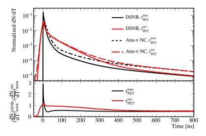
**Figure 5.** The averaged true (black) and reconstructed (red) profiles of the photon emission time (PET) are illustrated for both the DSNB signal (solid) and NC background (dashed). The upper panel is shown for the normalized time profiles and the lower panel for the relative ratios of the DSNB signal and NC background.
