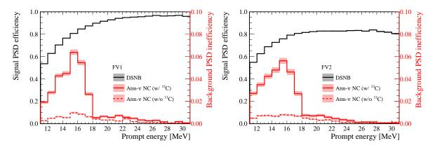
Figure 6. PSD efficiencies as functions of the prompt energy with the BDT method. The left and right panels are shown for the signal and background efficiencies in the regions of FV1 and FV2. The black solid lines are for the signal efficiency after the PSD cut, and the red lines are for the background inefficiencies of the atmospheric  $\nu$  NC backgrounds with (solid) and without (dashed) <sup>11</sup>C. The shadowed bands are shown for the statistical uncertainty of simulated data samples.
