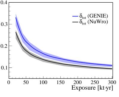
Figure 4. The relative uncertainty of the NC background as a function of the detector exposure by taking account of the envisaged *in situ* measurement at JUNO. The bands are obtained by assuming different levels of natural radioactivity and cosmogenic <sup>11</sup>C in the accidental background.
