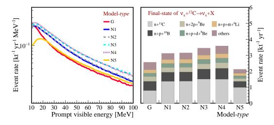
**Figure 3**. Left panel: event rates of the NC background as a function of the prompt energy using six different neutrino interaction models. Right panel: event rates of the NC background for specific channels with different final-state nuclei in the prompt energy range from 12 to 30 MeV.
