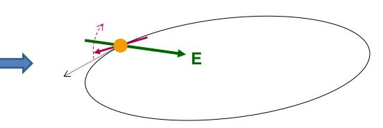
Polarization starts parallel to velocity, rotates toward vertical due to E-field. Look for the change.
