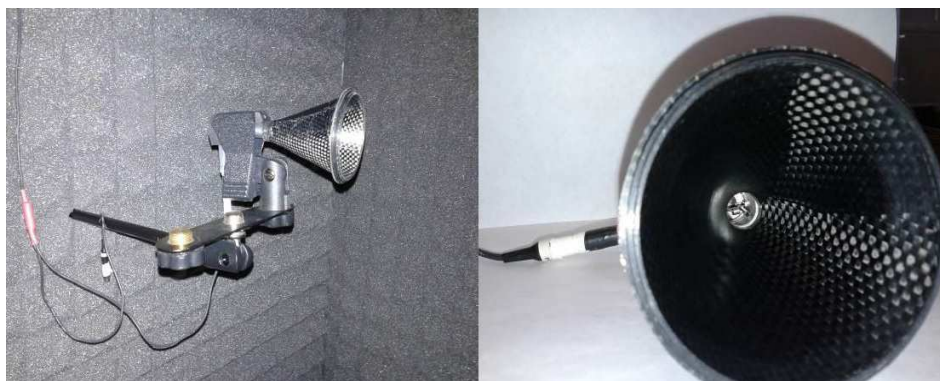
Figure 1- Horn made of carbon fibre applied to the p-v probe.
