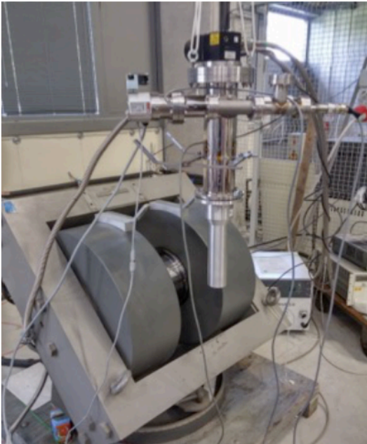
MgB2 trapped magnetization after transition to superconductor
