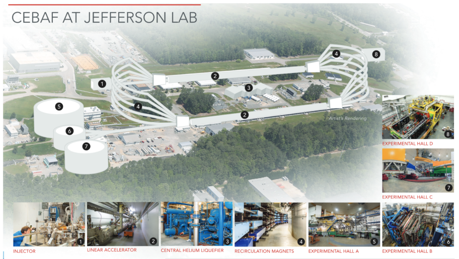
Figure 2.2: The CEBAF and experimental halls scheme
