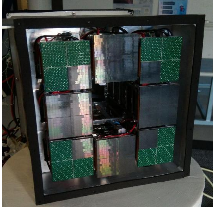
(a) Picture of the photo-detector side of the SiPM detector box.
