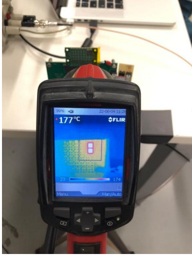
(a) Picture of the thermal camera measuring the directly polarized SiPM. It can reach more than 175 °C.
