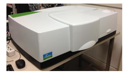
The uncertainty assigned to the spectrophotometer measurements takes into account the spread of T values obtained by illuminating 6 different positions of a given tile:
