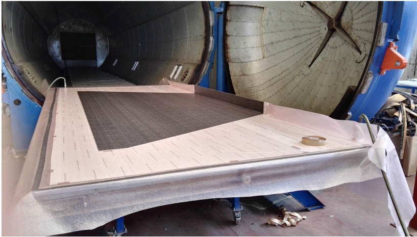
3m diameter autoclave housing large panels
