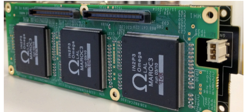
3 x ASIC BOARD (INFN) matching the
