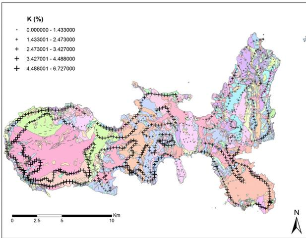
Fig. 2. Geological map of Elba Island (derived from the new Geological Map of Tuscany region realized at 1:10,000 scale by CGT, 2011). The measurements of potassium concentration are reported (crosses). For the complete official legend of the whole geological formations see [159.213.57.103/geoweb/10k/legenda10ktoscana.pdf](http://159.213.57.103/geoweb/10k/legenda10ktoscana.pdf). The coordinate system is UTM WGS84 Zone 32 North.
