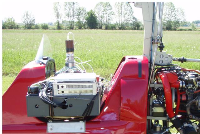
Fig. 1. The AGRS system mounted on the vehicle.
