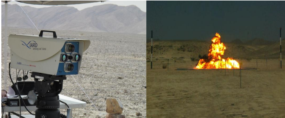
Figure 1: The IARD ColoRad C7 (right) and high speed fireball snapshot 10 ms following TNT detonation
