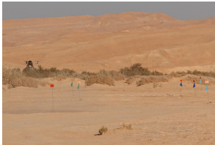
Figure 1: Mikro-Kopter / multi-rotor (upper) Airborne radiation survey of ^{99m}\text{Tc} from “Green field” (Open field) test compared with ground survey (lower) [2].
