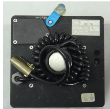
(b) The detector casing, Source B is encased in the detector.
