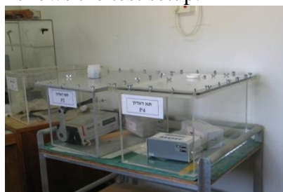
Figure 2. Setup for radon exhalation measurements using the sealed chamber method.
