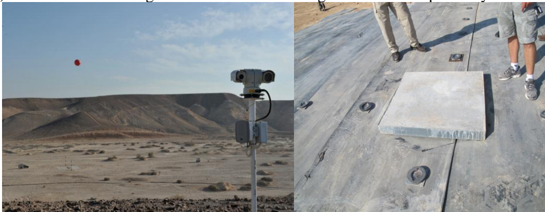
Figure 1: The GZ area (on concrete surface - right) and far field look (left) of the test site. Height reference balloon and a video camera are on the left.
