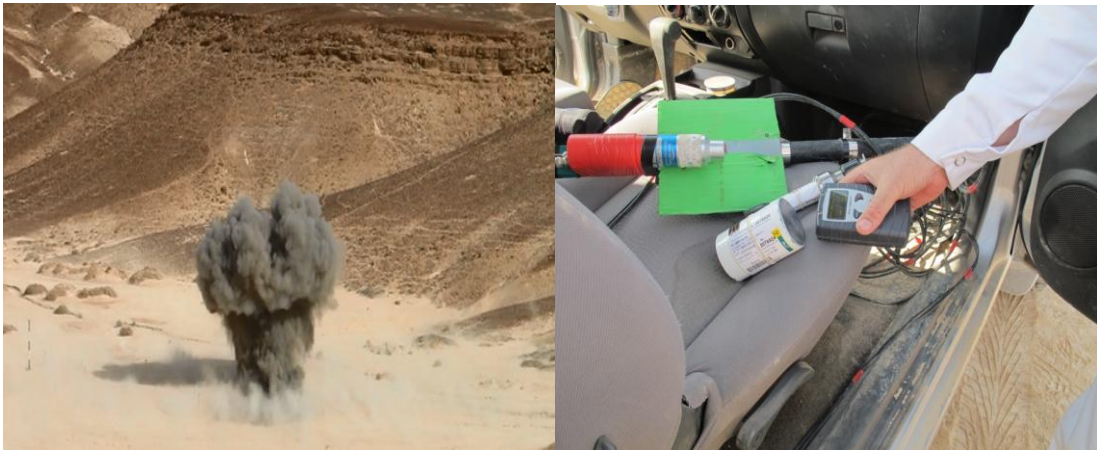
Figure 2: Portable \text{LnBr}_3 detector with a lead shield plate and a PDS (right) and 25 kg of TNT cloud 4 s following the detonation (left).
