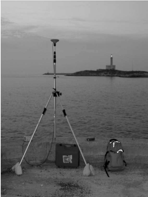
Figure 2: DGPS measurement at 157701 IGM95 vertex (Vieste, S.Francesco Church).
