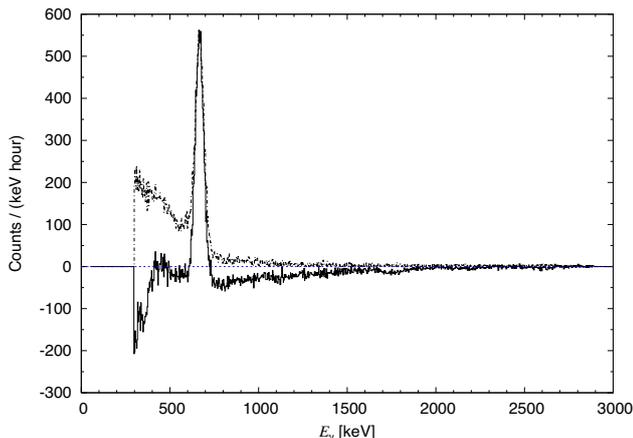
Fig. 1. The reconstructed sensitive spectrum for  $^{137}\text{Cs}$  by using simple FSA (full line) and FSA+NNLS (dot dashed line). By implementing the NNLS constraint the non physical effects disappear.
