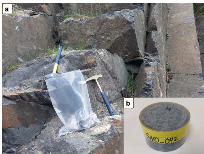
Figure 3. Rock sample of lapilli tuff (Geocode 28c, Onaping Fm.). (a) Each sample was collected from fresh outcrop and (b) then crushed and sealed in polycarbonate box of 180 \text{ cm}^3 of volume.
