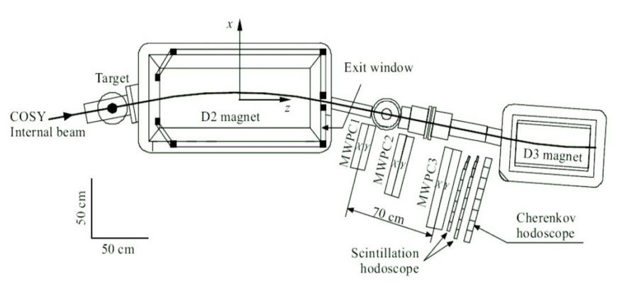
1<sup>st</sup> version MWPC1, MWPC2, MWPC3: X1,strip,Y1,strip pitch ~ 1mm -> resolution RMS ~0.3 mm
