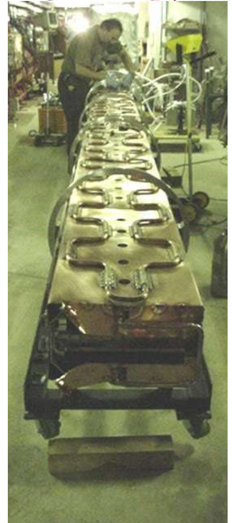
Pickups cooled by Liquid Nitrogen
