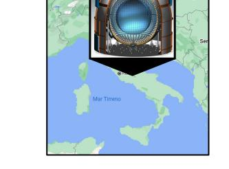
**Borexino** is **0.3 kton** liquid scintillator detector situated in **Italy**, at the Laboratori Nazionali del Gran Sasso. It is surrounded by ~2200 8" PMTs.
