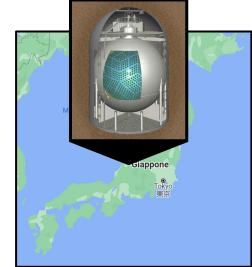
**KamLAND** is a **1 kton** liquid scintillator detector situated in Japan, in the Kamioka mine. It is surrounded by 1325 17" PMTs and 554 20" PMTs.
