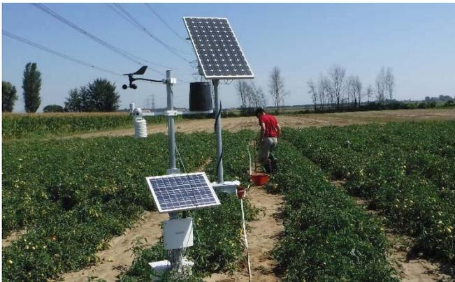
Fig. 2. The agro-meteorological station (in the foreground) and the PGR station (in the background).
