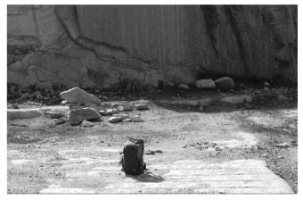
*Fig.* I – Portable gamma-ray spectrometer in a quarry during the acquisition of K-U-Th isotopic concentration.
